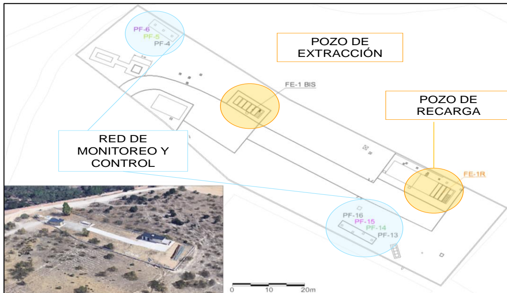
Figure 4. ASRT outdoor and floor ASRT facilities.
