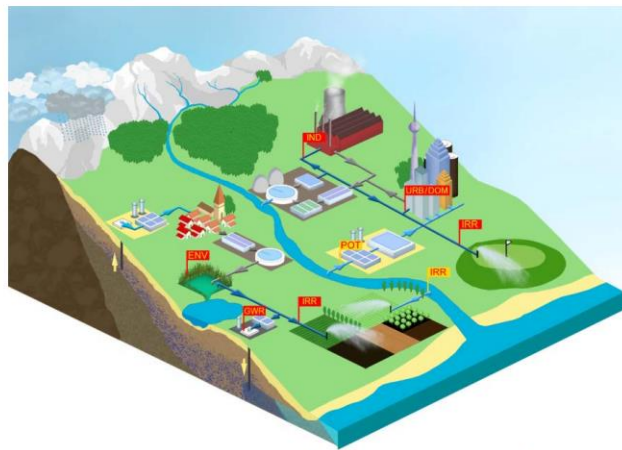
Figure 8.1 The anthropogenic water cycle with direct and indirect water reuse (modified from Veolia Water, Durham 2005, where : indirect reuse : direct reuse, GWR: groundwater recharge, IRR: irrigation, POT: potable reuse, IND: industrial reuse, URB / DOM: urban & domestic reuse, ENV: environmental enhancement)
