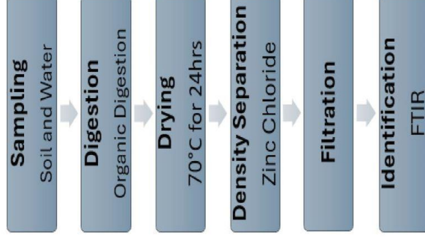
Figure 3: The process of acquiring data, from sampling, sample preparation, to analysis, and identification of MPs
