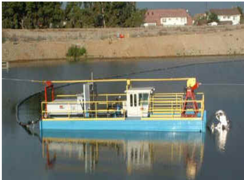
Figure 3-9. Example for a Basin Cleaning Vehicles (BCV) in Holland.
