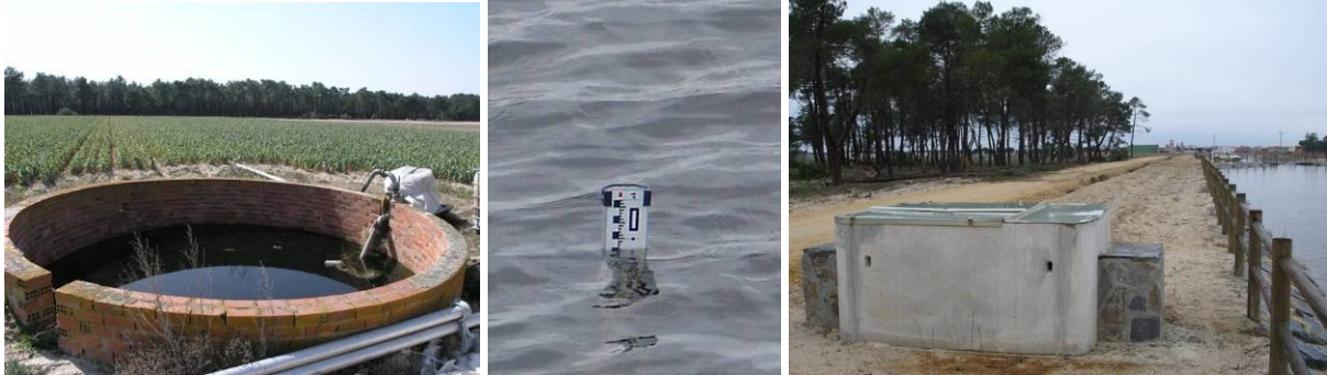
Figures 5-28 a) to c) Some examples for technical solutions already deployed in Arenales Aquifer, Spain. MAR Well connected to the canal used for water management (a), water layer thickness controlled in infiltration ponds (b), and MAR management by valves / flow meters (c).
