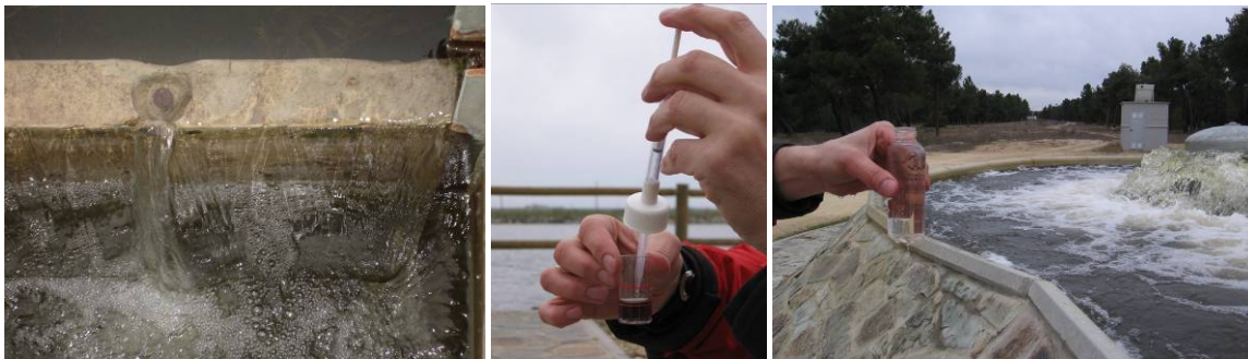
Figures 5-16 a) to c). Recharge water with 7.5 ppm of total dissolved oxygen, in situ determinations and sample collection.
