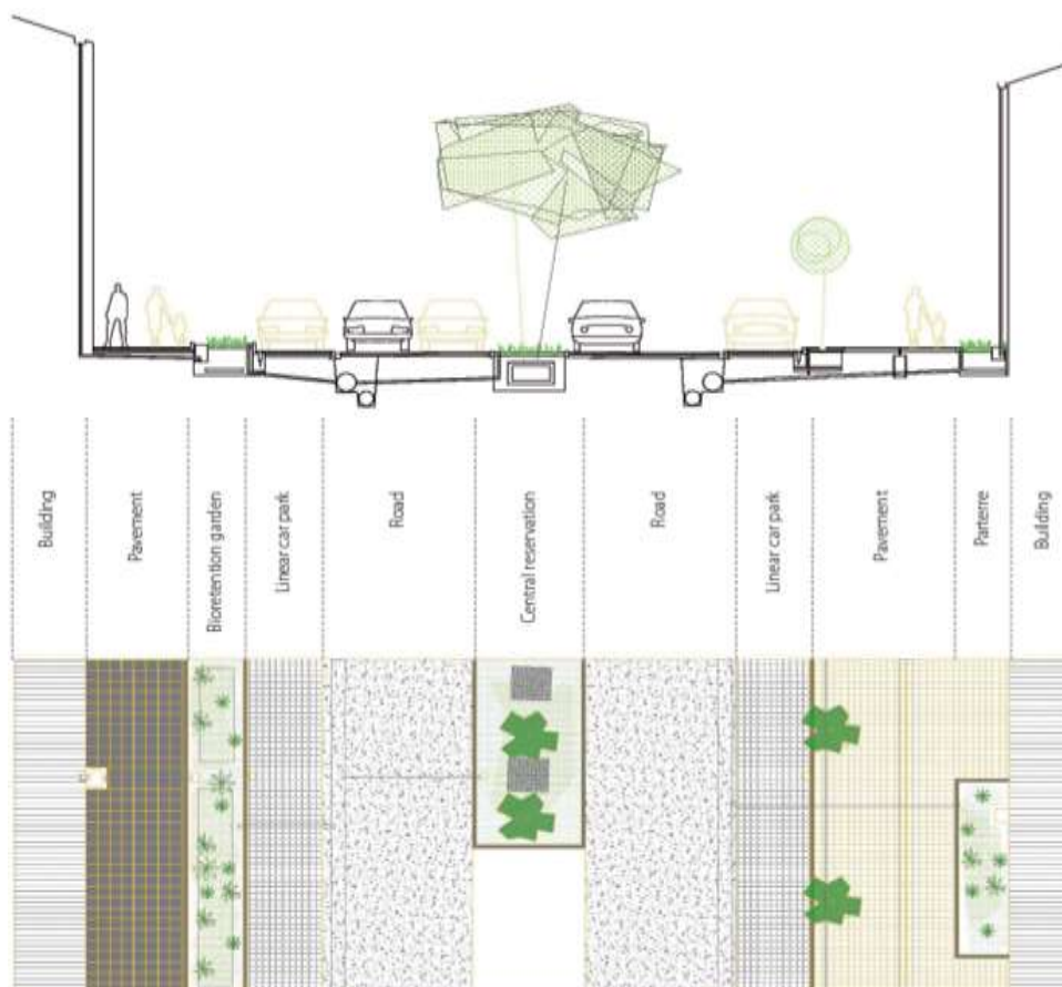
Figure 4-73: Detail of the cross section and plan for an average width street. Extracted from GIAE (The Comprehensive Management of Rainwater in Built-up Areas), Tragsa Group, 2015.
