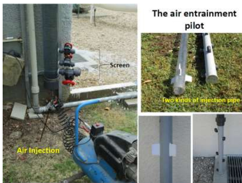
Figures 4-55: Air entrapment pilot in Menashe demo-site (Israel). Courtesy of Mekorot. co.
