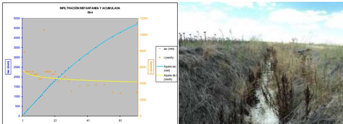
Figures 3-3 a & b: Infiltration rate test charting conducted at the MAR canal (a). Vegetated canal bed showing whitish crust (b).
