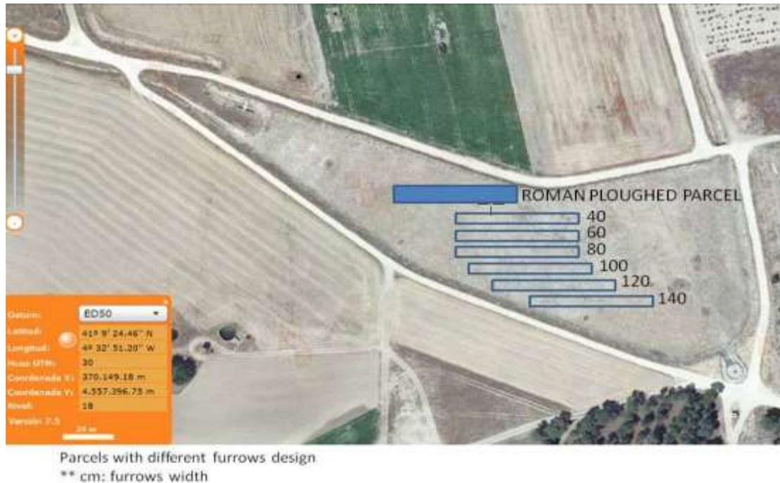
Figure 3-4: Santiuste Basin's head infiltration pond with seven parcels furrowed with a different width.
