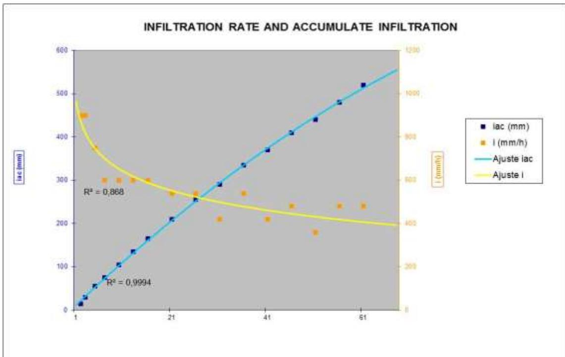
Figures 3-12 a to d: Infiltration test (a-b), soil profile (top at the right side) (c), and result for the vegetated location (d).
