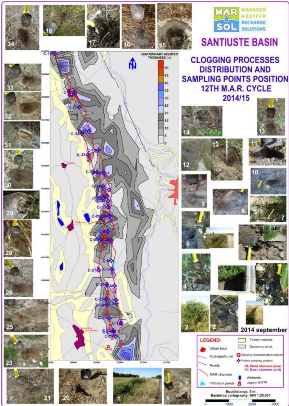
Figure 3-23: Network to study the clogging processes at Santiuste basin MAR system, and sampling/data collection for the situation of 2014 September.
