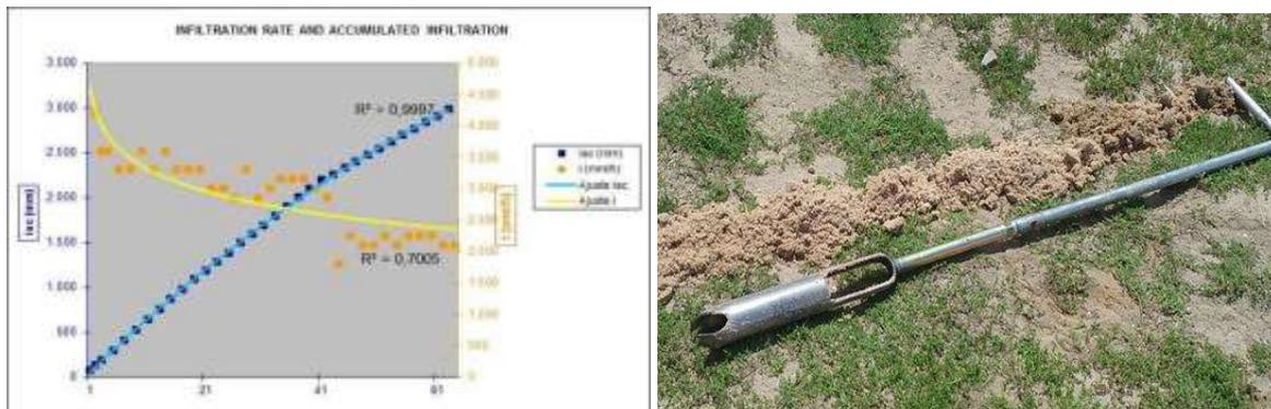
Figures 3-6 a & b: Infiltration test chart for the pond analysis furrowed 40 cm spacing (a) and soil profile with the bottom at the left hand (b).
