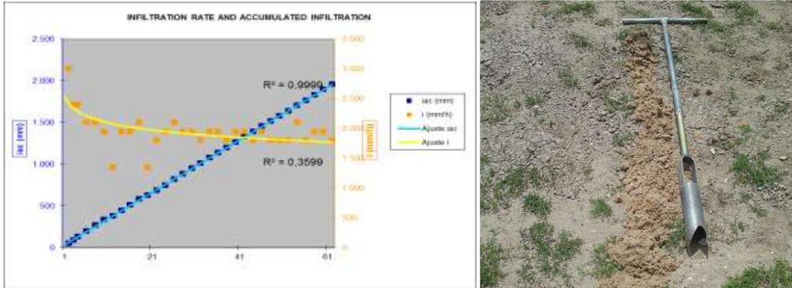
Figures 3-7 a & b: Infiltration test chart for the pond analysis furrowed 140 cm spacing (a) and soil profile with the top at the upper side (b).
