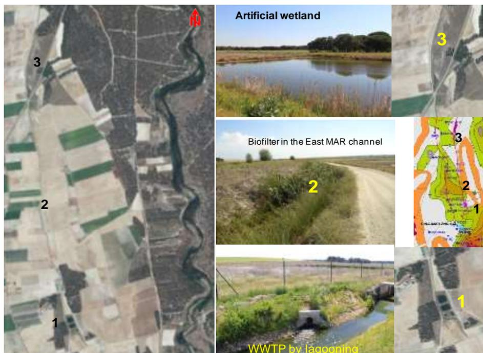
Figure 3-32: “Triplet” at Santiuste basin, a combination of elements to play a purification process on reclaimed water from a lagooning WWTP: spill of reclaimed water in the MAR canal (1); natural treatment along a green biofilter (2) and final treatment along two artificial wetlands (3).
