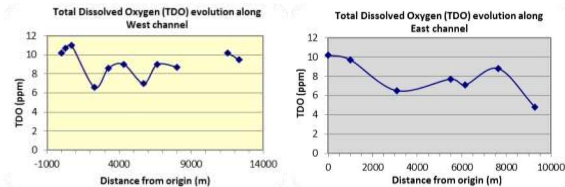
Figures 3-24 a & b: TDO evolution representation along the MAR channels West (a) and East (b).
