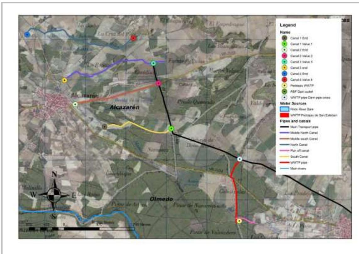
Figure 3-43: Alcazarén area. Cartographical mock-up for the MAR facilities in the area.
