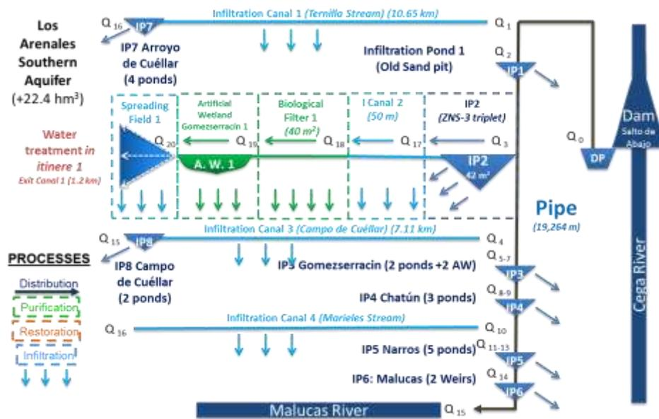
Figure 3-35 Operational sketch of El Carracillo MAR plant. The *triplet* is situated at IP3.
