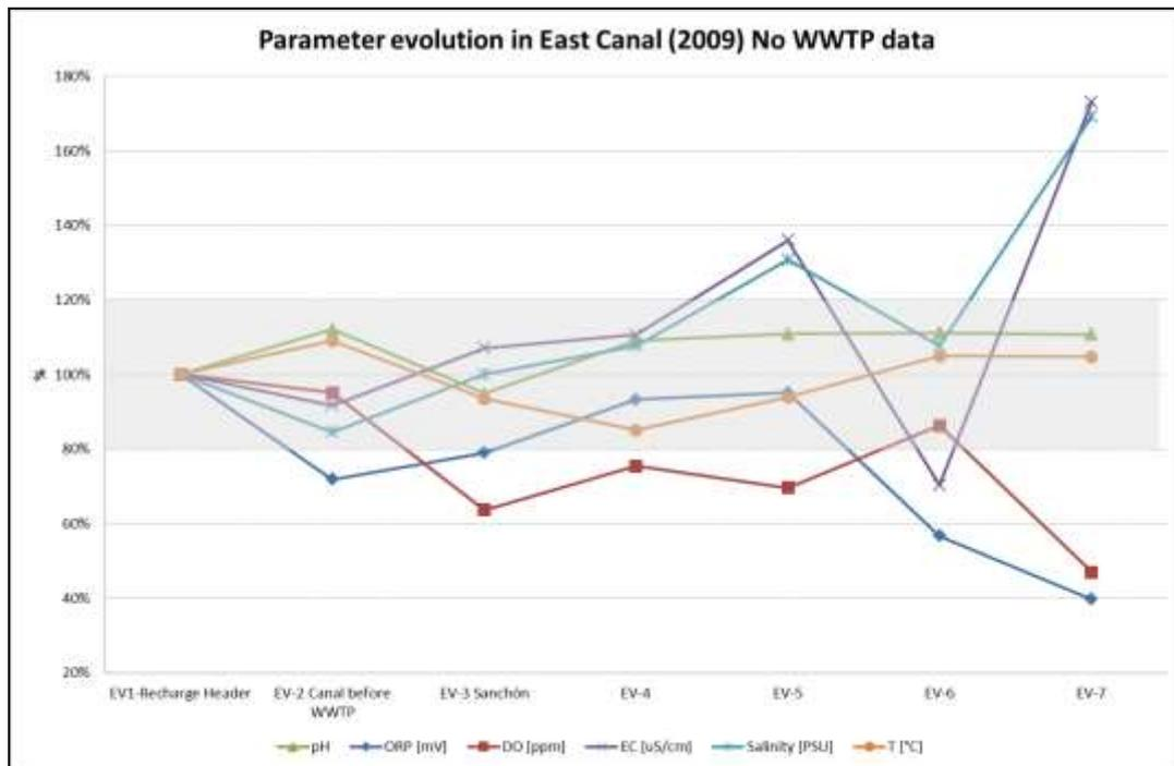
Figure 3-39: Unstable parameters evolution graph in Santiuste triplet (2009).
