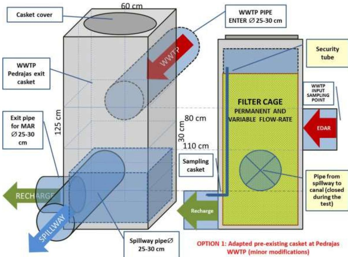
Figure 3-46: Initial filter casket with slight modifications
