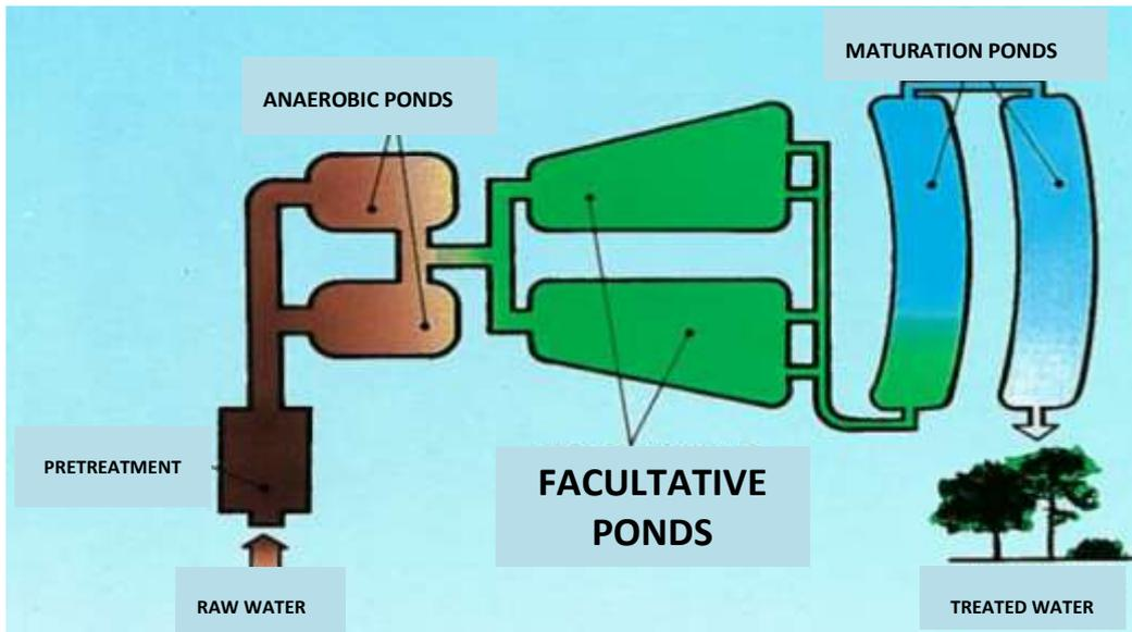
Figure 3-57: Most common scheme used in the natural lagooning.
