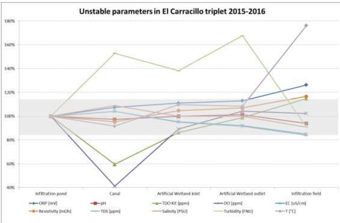
Figures 3-42 a & b: Unstable parameters evolution graph in El Carracillo triplet (2015-2016).
