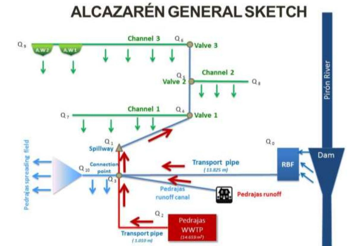
Figure 3-44: Alcazarén area general sketch where the conductions and piping tests have taken place. Topologic scheme.
