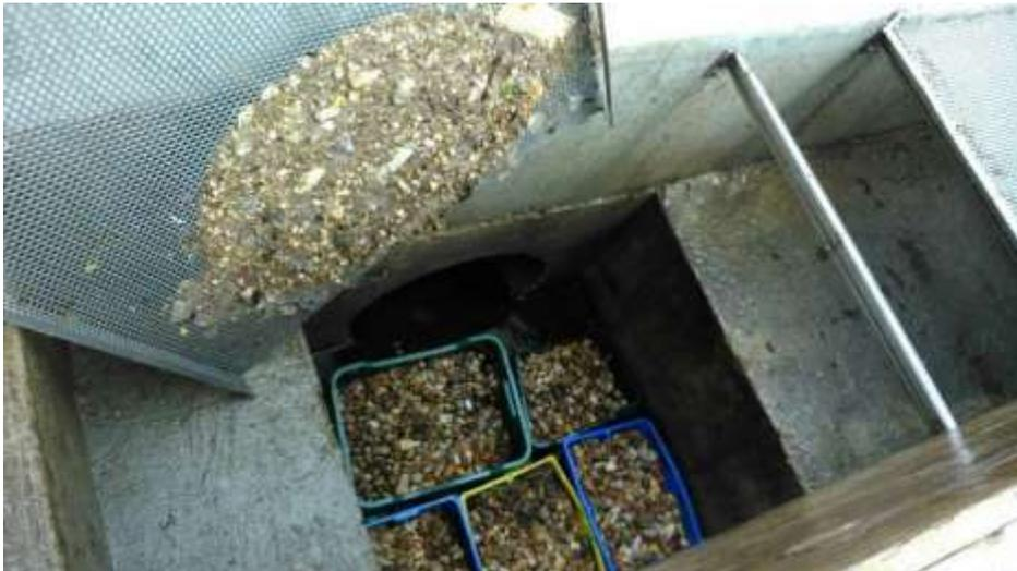
Figure 3-50: Alcazarén area. Test with an inorganic siliceous gravel filter combined with a metal grid in the final testing area 100 m downstream the WWTP.
