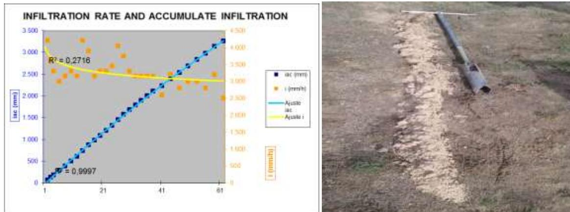
Figures 3-8 a & b: Infiltration test chart for the pond analysis furrowed 80 cm spacing (a) and soil profile with the top at the upper side (b).
