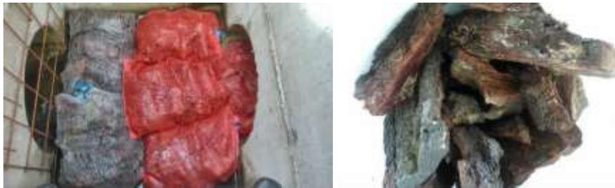
Figure 3-52: Alcazarén area. Test with an organic reactive layer (pine bark filter).
