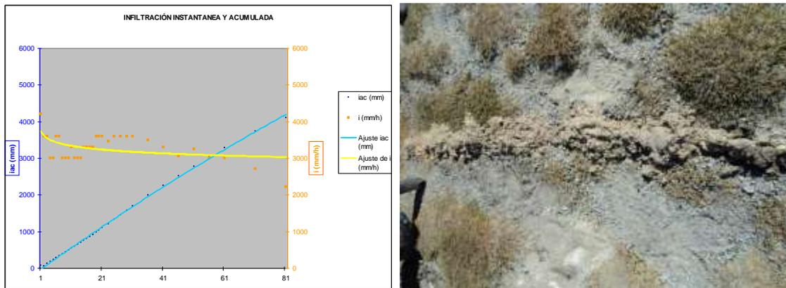
Figures 3-2 a & b: Infiltration test chart for the pond analysis (a) and soil profile with the bottom at the left hand (b).
