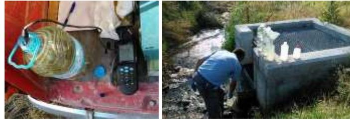
Figure 3-55: Alcazarén area. DBP test dropping hypochlorite at the exit of the WWTP and samples collection.
