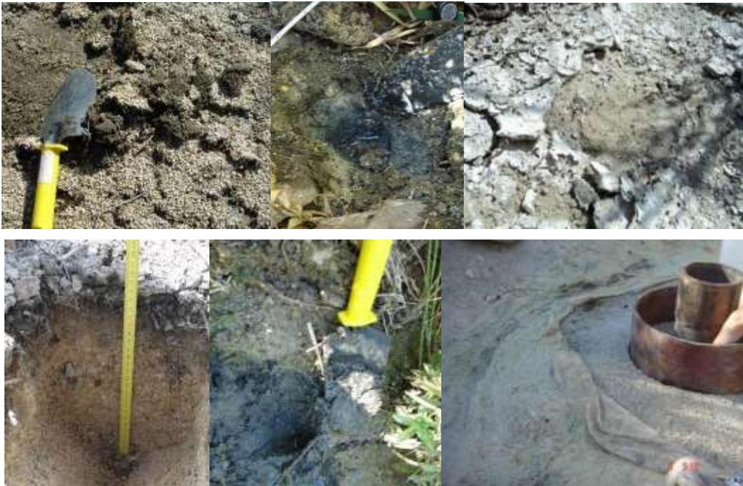
Figures 3-22 a to e: Physical clogging processes (a); biological and biophysics (b); chemical processes (carbonates) (c); vegetated canal bed showing whitish crust (d); physical-biological (e) and biological (filamentous algae colonies) (f) observed at Santiuste basin MAR ponds and canals.
