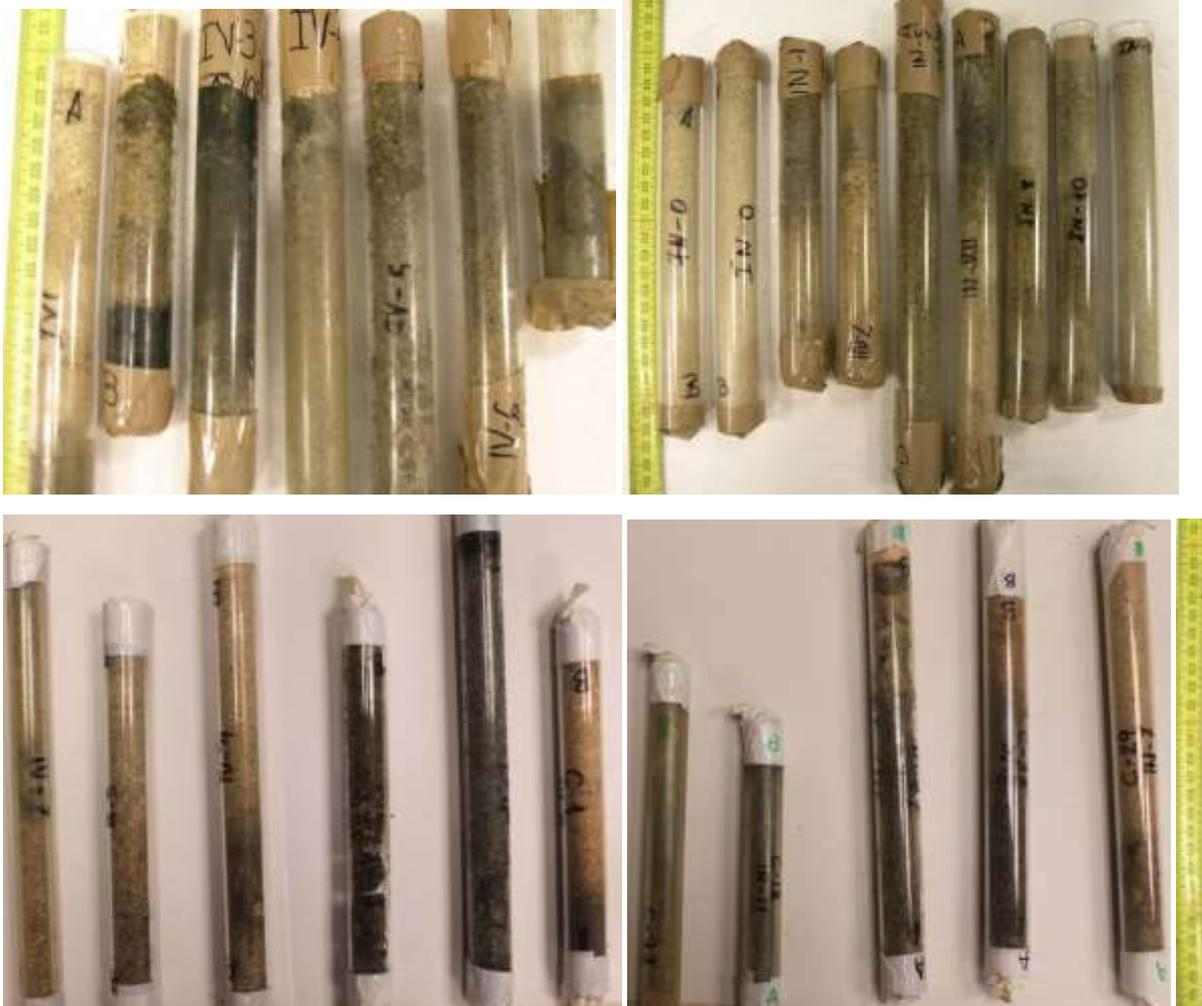
Samples of 2009 (up) and 2015 (below) so as to compare the clogging profile.
