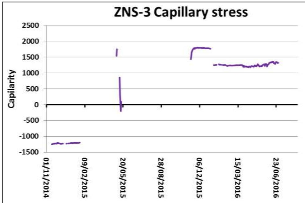
Figure 3-28: Capillary tension chart showing the evolution registered at MARSOL ZNS 3 Station between 2008 November and 2016 June. Sensor installed 1.5 m depth.
