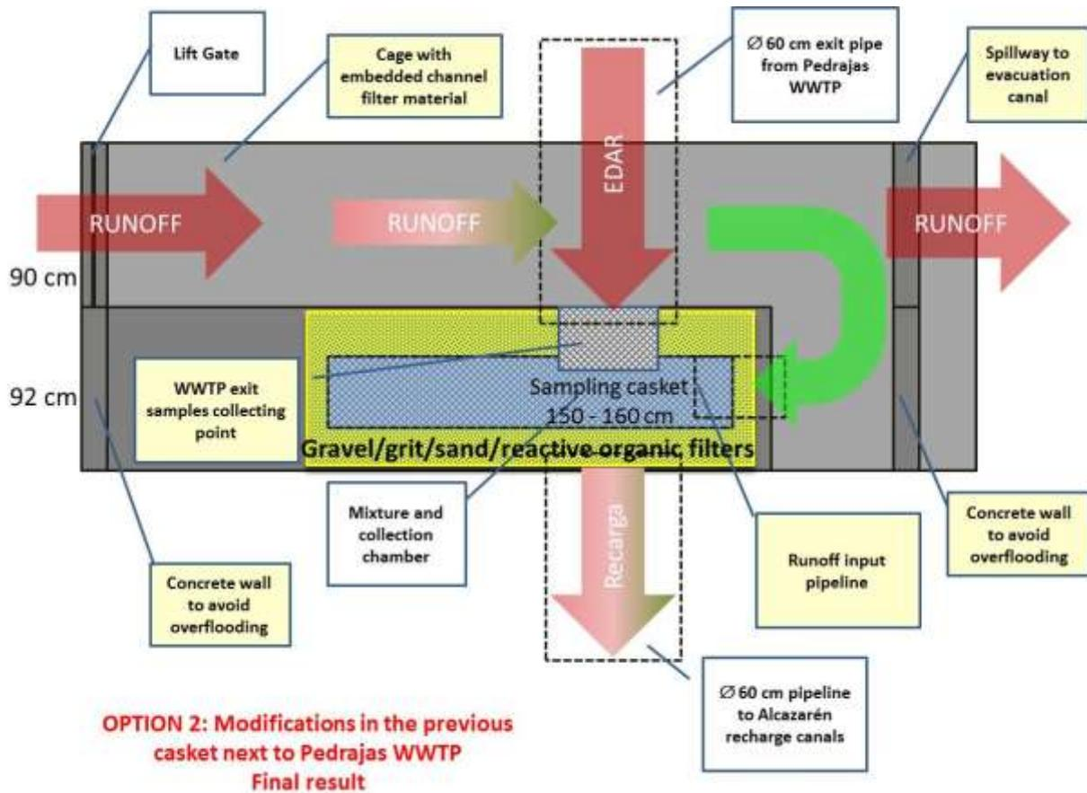
Figure 3-48: Specific system to perform the tests constructed in the point where the three different water sources converge.
