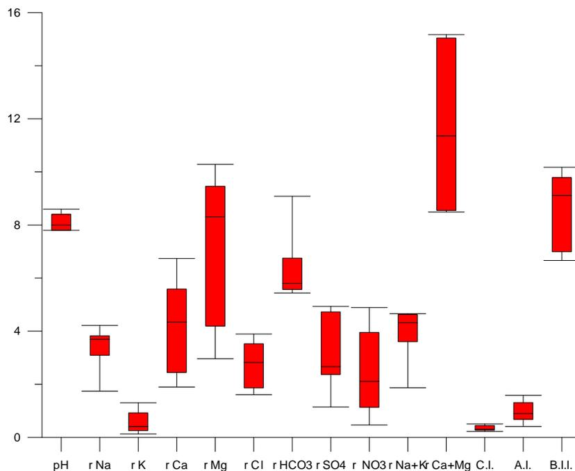
Figure 3-31: Box-plot charting all the analysed wells for 15 chemical parameters.
