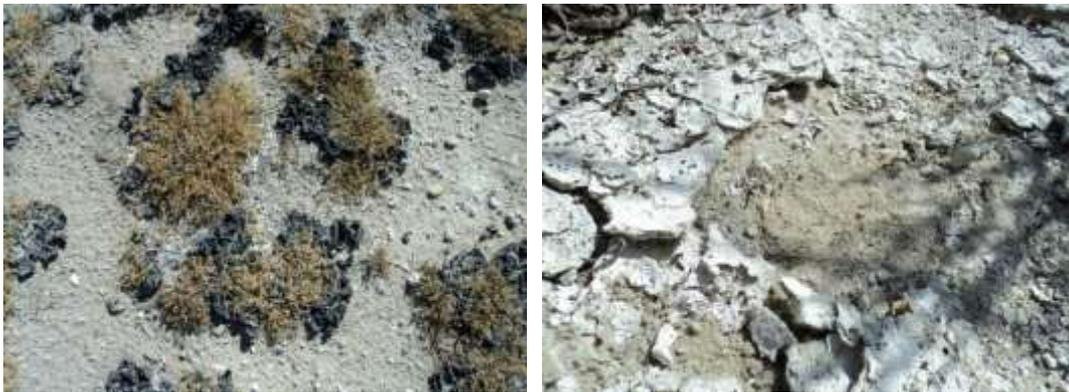
Figures 3-18 a & b: Dark organic patches (a) and whitish crust on infiltration surface (b) at Santiuste MAR canal.
