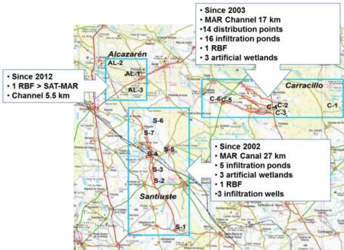
Figure 3-1: Los Arenales aquifer MAR systems position and devise of the facilities on the topographic map with a list of the main MAR components. Approximate scale: 1:150.000.
