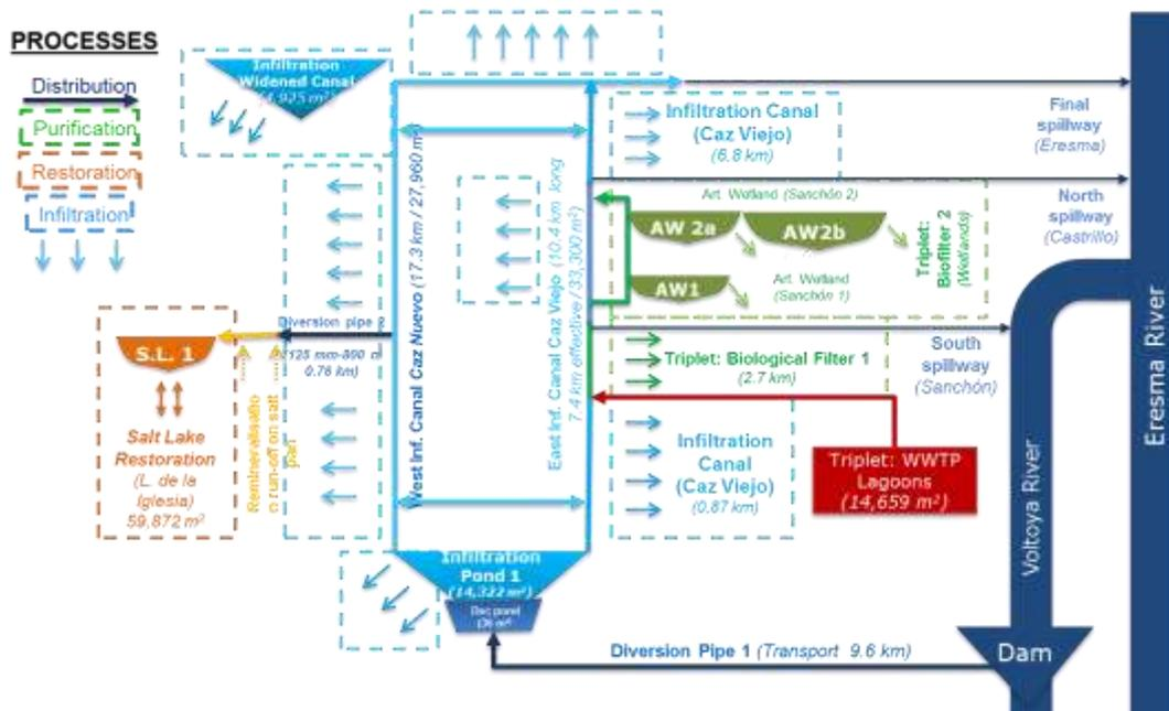
Figure 3-21: Operational sketch of Santiuste basin, the pioneer MAR plant at Los Arenales aquifer.
