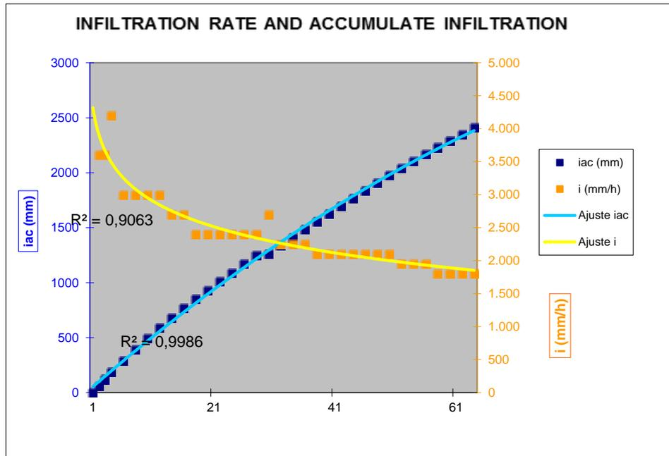
Figure 3-9: Infiltration test chart for the pond unaltered area.
