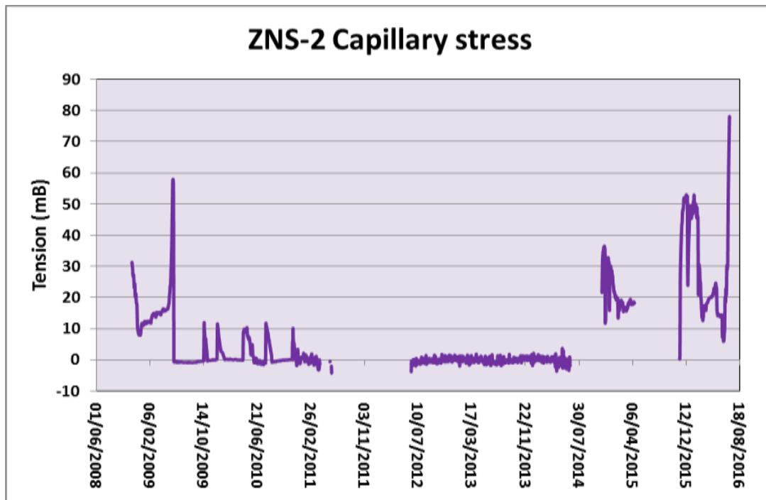
Figure 3-27: Capillary tension chart showing the evolution registered at MARSOL ZNS 2 Station between 2008 November and 2016 June. Sensor installed at 1.2 m depth.
