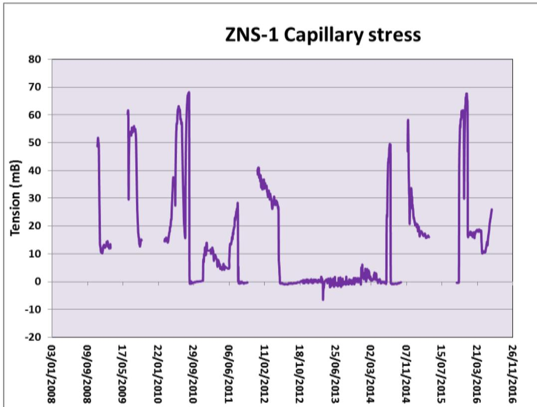
Figure 3-26: Capillary tension chart showing the evolution registered at MARSOL ZNS 1 Station between 2008 November and 2016 June. Sensor installed 1.2 m depth.
