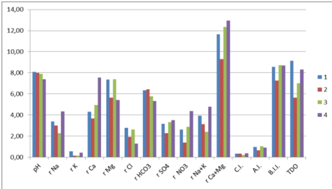
Figure 3-30: Histogram charting all the analysed wells (mean values) grouped according to their associated clogging processes.
