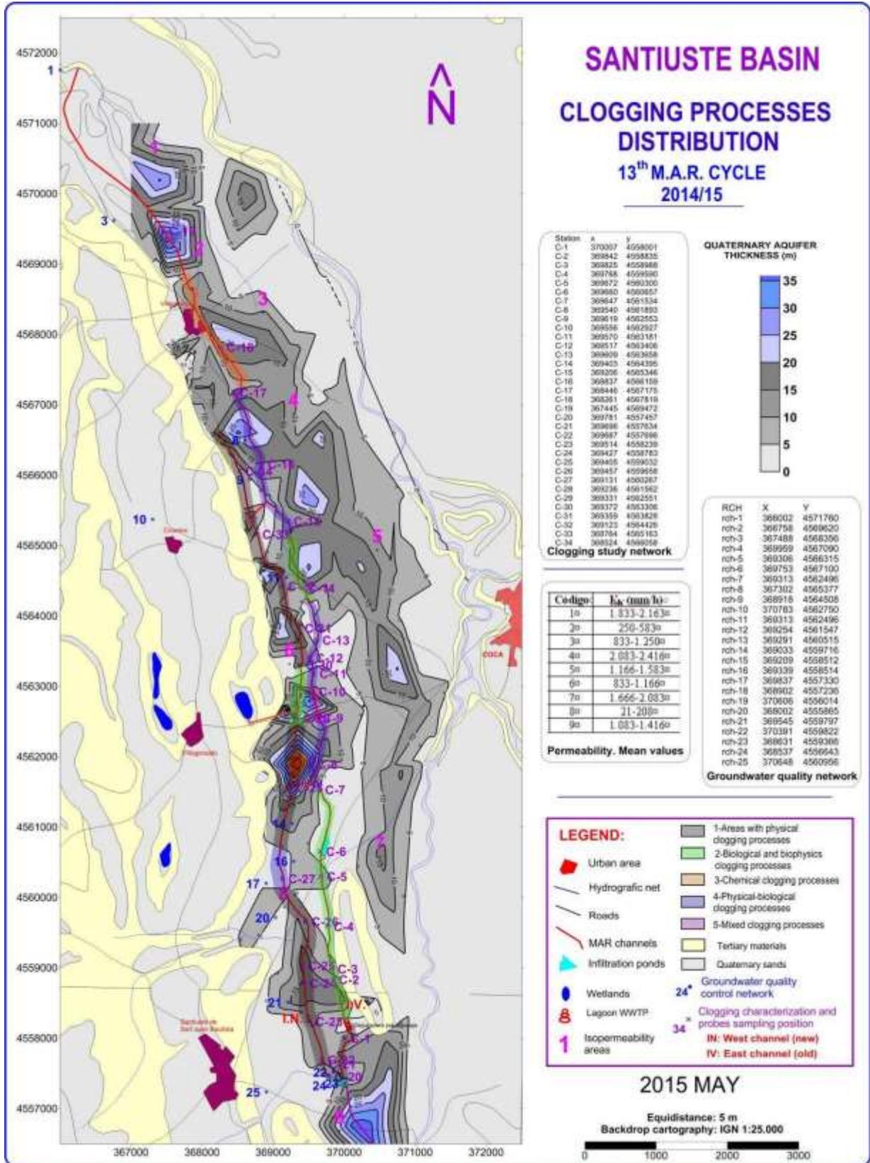
Figure 3-29: Cartography for Santiuste basin MAR devices and clogging processes distribution according to their nature for May 2015 situation. The map also exposes geological facies, the position of clogging stations, groundwater quality network, permeability distribution in the area and other singular elements. Graphic scale (Modified from MARSOL, 2015a).
