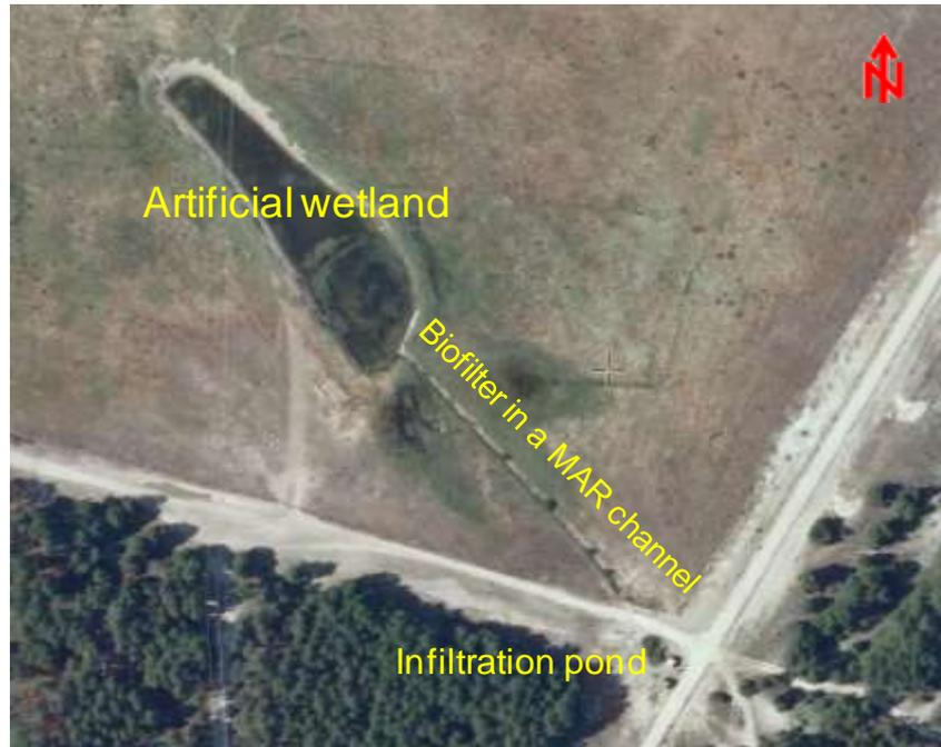
Figure 3-36: El Carracillo “triplet” components: stagnation strainer and infiltration pond (1), green biofilter along the MAR canal (2) and artificial wetland (3) with a spillway directed northwest wards to a spreading field for MAR.
