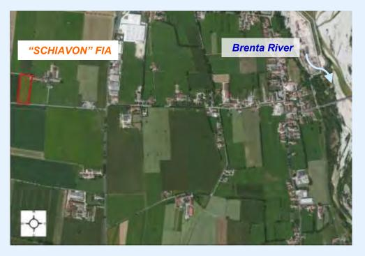
The watering of the pilot F.I.A. area takes place generally during non-irrigation periods, using the existing irrigation water conveyance system (**ditches, underground pipelines**). Approx. 2 hectares
