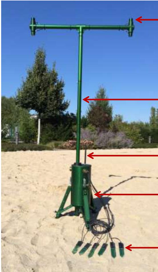
Optical sensors: photosynthetically active radiation (PAR) and 4 wavelength specific sensors (net balance)
