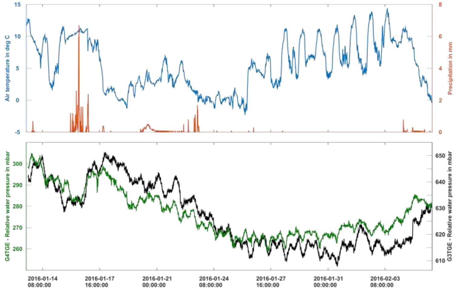
Exemplary measurement results from the wireless sensor network in Lavrion
