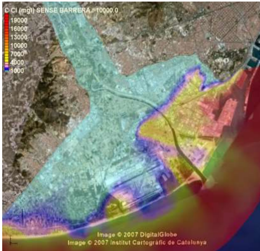
WITHOUT Hydraulic barrier
