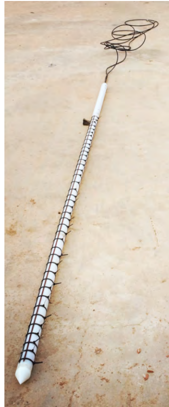
Preparation of FD-sensor rode with cables for two side measurements
