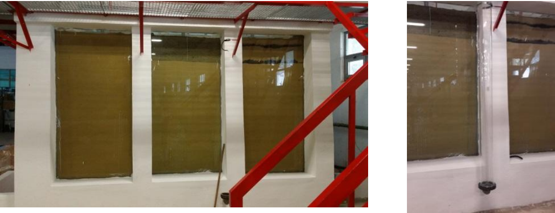
Figure 100 – Detail of three soil layers being tested simultaneously (left) and the external piezometer (right)
