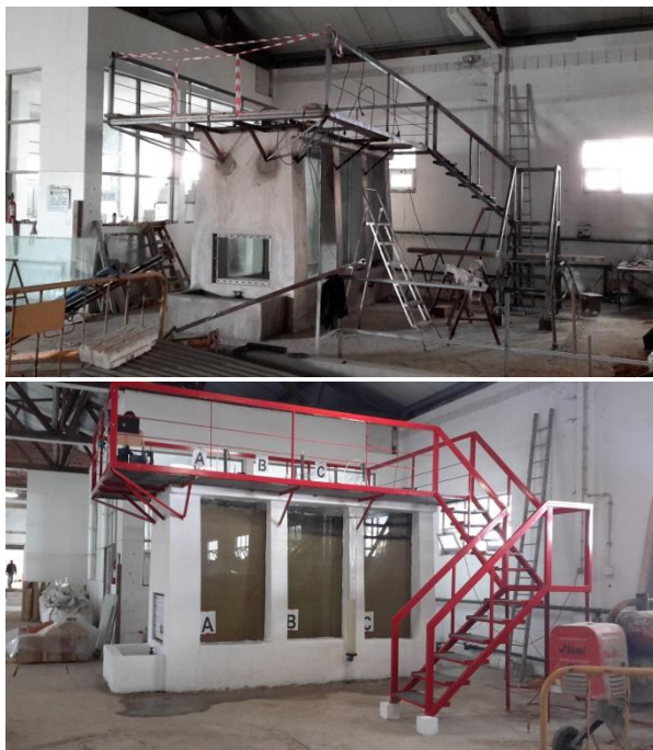
Figure 98 – LNEC physical (sandbox) model construction
